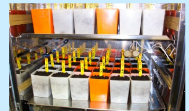
Experiment to determine the effect of A. bisporus on prochloraz degradation in a controlled environment cabinet
